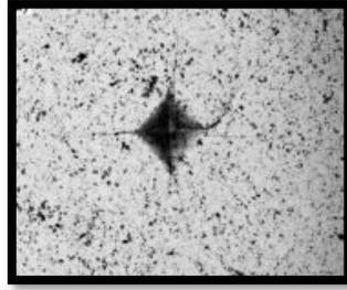
Fig 2- Indentation at 40× magnification measured using Vickers micro hardness testing machine
