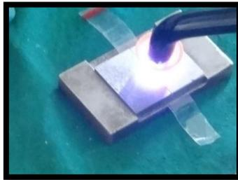
Fig 1- Mylar strip used to ensure smooth surface of the specimen.
