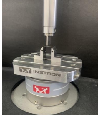
Figure 1: The above picture shows the esthetic arch wire specimen being tested on the Instron E3000 universal testing machine before application of force.
