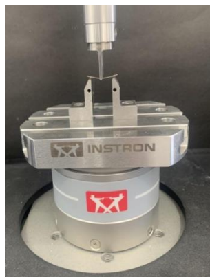
Figure 2: The above picture shows the esthetic arch wire specimen being tested on the Instron E3000 universal testing machine on application of force.
