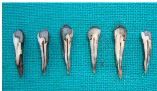
FIGURE 3 The teeth were sectioned bucco-lingually in to two portion to observed the microleakage at tooth-composite interface
