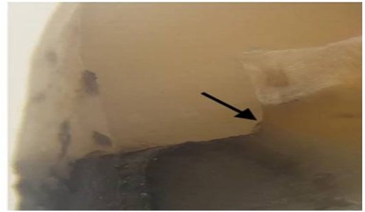
FIGURE 7 Dye penetrated from the edge of the materials to deeper depth
