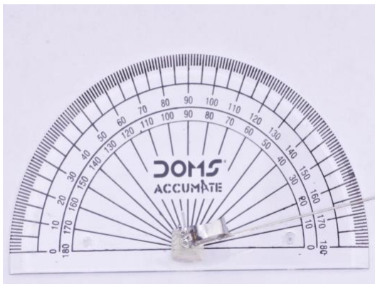
FIGURE 2 B. Bracket - arch wire play measurement (minimum play)
