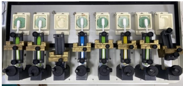
Figure 2: Tooth brushing simulator (ZM-3.8, SD Mechatronik, Germany)
