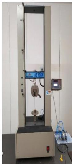
Fig 3: Universal testing machine-
