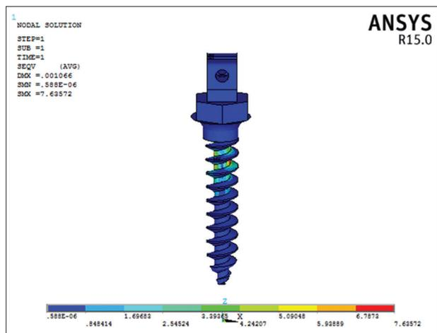
Figure 4: Stress generation on the implant for the given load of 150 g
