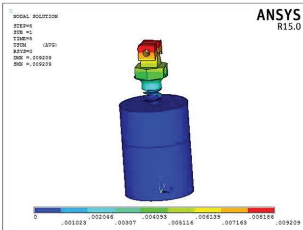
Figure 3: Displacement of implant with application of 150 g force to 3 mm thick cortical bone
