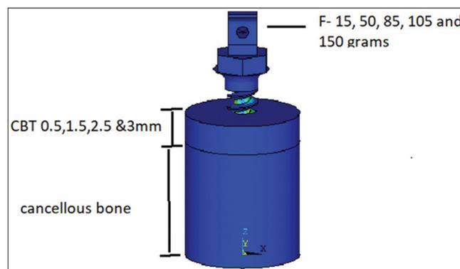
Figure 1: Geometric assembly of OMI and bone specimens used in the study after meshing step
