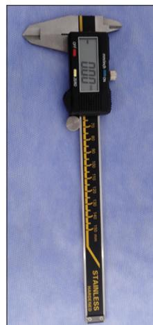
Figure 1: Digital caliper used for measuring tooth width
