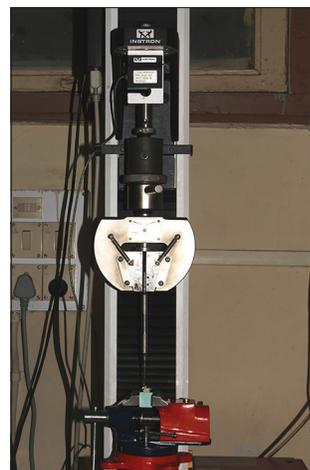
Figure 10: Shear bond strength test using universal testing machine
