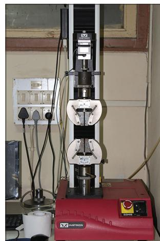
Figure 4: Universal testing machine (Instron)
