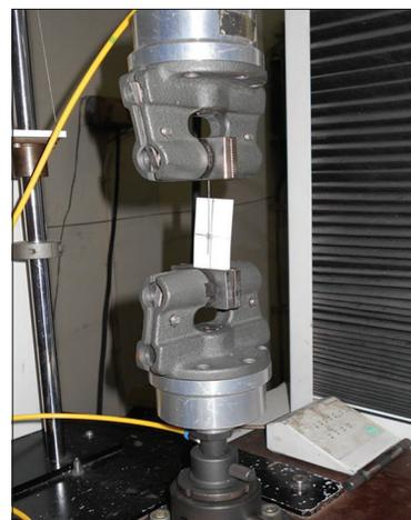
Figure 1: Universal test machine with the sample mounted for testing
