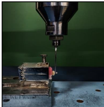
Fig 7: Testing of shear bond test
