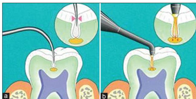
Figure 10: (a and b) DIAGNOdent mechanism.
