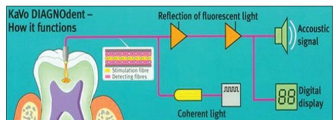
Figure 9: DIAGNOdent - laser autofluorescence.
