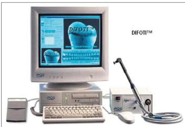
Figure 6: Digital imaging fiber-optic transillumination.
