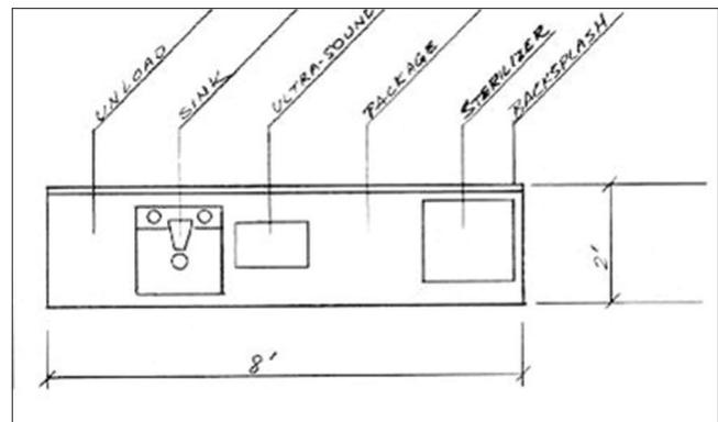
**Figure 2:** Schematic representation of sterilization room.
