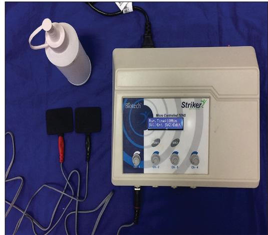
**Figure 2:** Assembly of TENS system.
