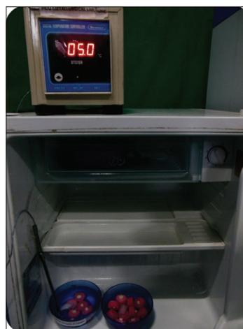
Figure 2: Thermocycling of samples.
