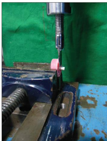
**Figure 6:** Evaluation of shear bond strength by universal testing machine.
