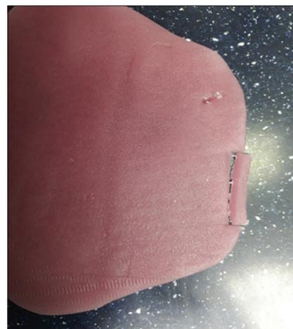
Figure 4: A bar of 16-mm length was cut from LCAR sheet by spatula.
