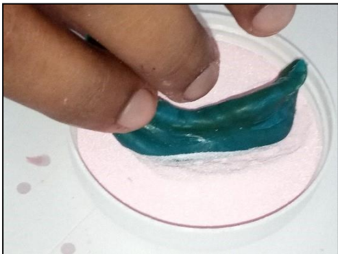
Figure 3: Dabbing / Dusting the monomer with polymer powder to allow it to stick on and polymerise
