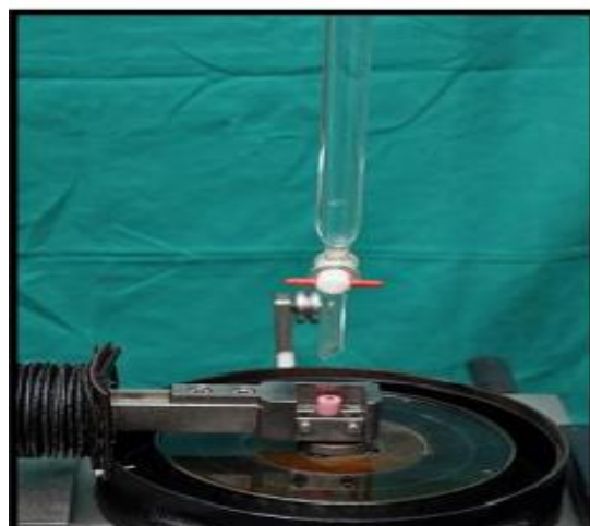
Figure 6: Wear test done under artificial saliva
