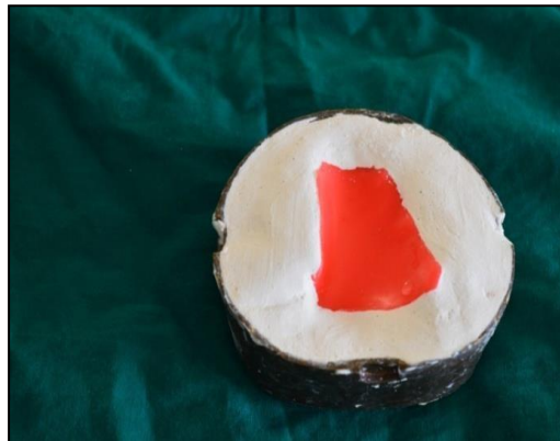
Figure 4. Part Flask used for fabricating Lid
